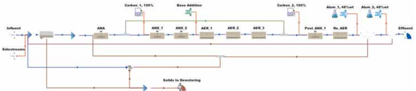
Figure 1. South Durham Water Reclamation Facility BioWin Flow Schematic
